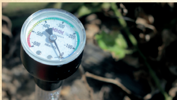
Tensiometers to measure soil moisture in Gastouni, Greece
